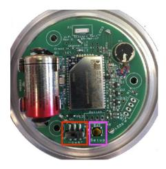
3. Within 30 secs of power on <u>carefully</u> press the <u>setup</u> button
